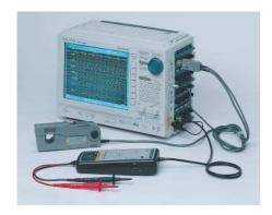
DL750 with current probe 701930 and differential probe 700924 connected.
